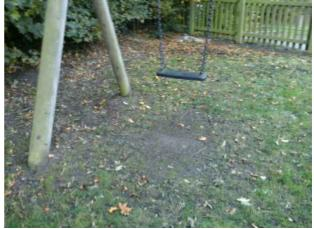
The grass mats are silted up and the soil is compacted; this may have an effect on the impact absorbing properties of the surface Finding:
